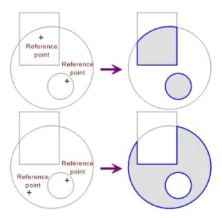
Reference point input is ended by clicking the right mouse button. Unlike most other commands, this does not lead to the previous entry being ignored; instead the command is processed with all previously entered reference points. If required, this can be undone using the <u>Undo</u> command.
