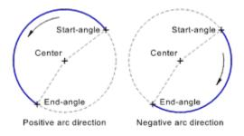
The appearance of the circular arc is shown during input, and changes if the current arc direction is changed.
