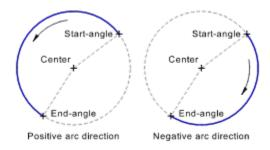
The appearance of the arc is show while it is being entered and changes immediately if the current arc direction is changed.
