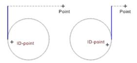
After identifying the object, a straight line appears which runs vertically and is tangent to the identified object.
