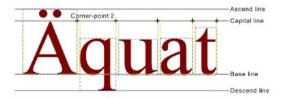
Optionally, specific coordinates can be entered. To do this, press the F8 key or ENTER. Absolute, relative or polar coordinates can now be entered. Relative coordinates relate to the first corner point. For further information on coordinate entry, see <u>Coordinate Entry</u> (F8).
