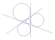
The 'right' circle can then be chosen with the help of the small dialog which appears at the bottom of the screen. Only one circle can be chosen at a time.
