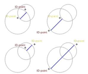
After determining the distance to be measured, the position of the dimension line and dimension text must be specified. To do this, several points have to be entered. How many, and which, points have to be entered, depends on the specified dimension parameters.
