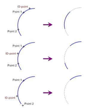
Note a basic rule for trimming: the object is always changed where it is clicked on!
